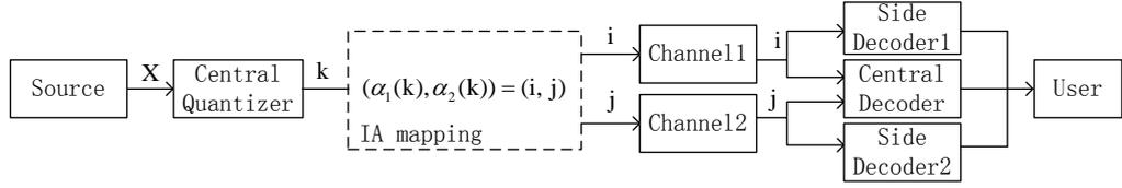
Figure 2.1: 2-DSQ system with two channels and three receivers
