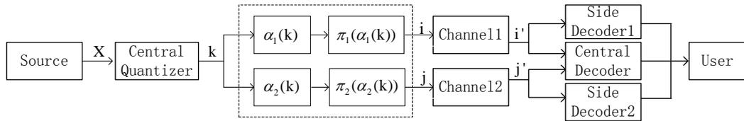
Figure 2.4: MDSQ system with bit-errors for two channels and three receivers
