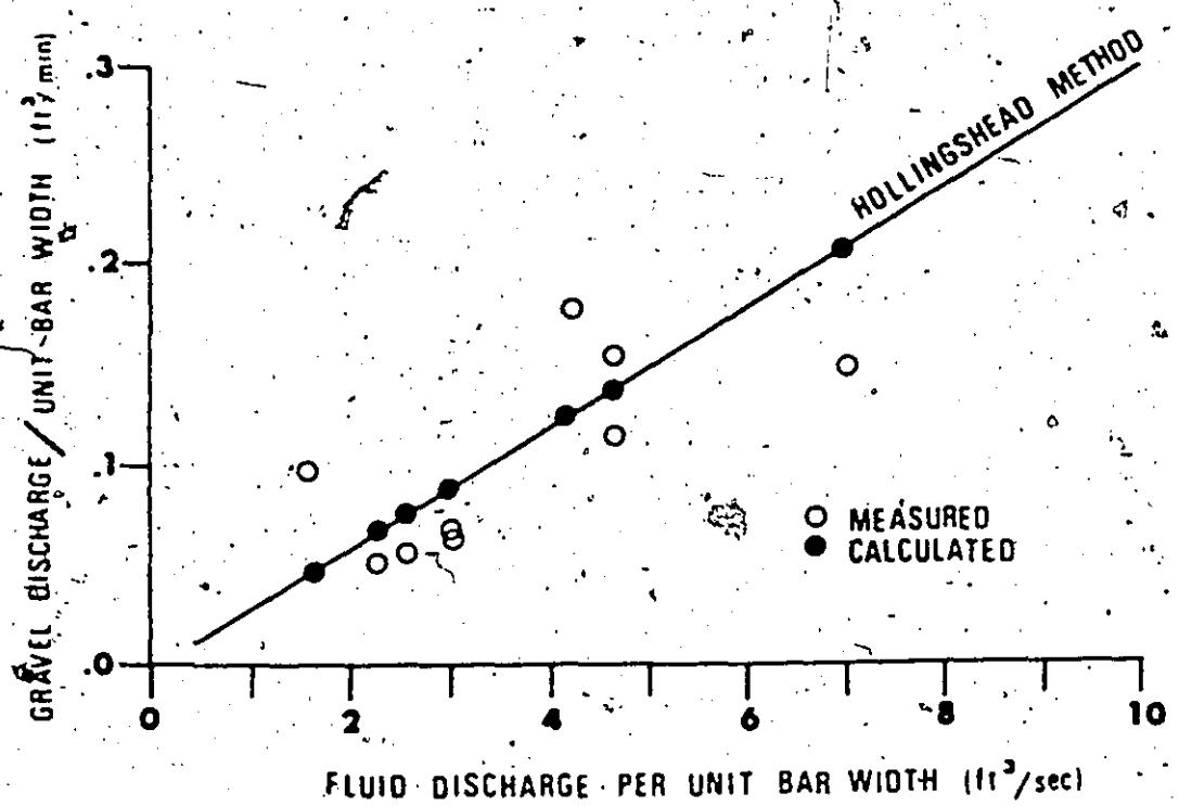
calculated as the product of bar height times bar advance rates. Gravel discharges per unit bar width ranged from  $0.052 \text{ ft}^3/\text{min}$  to  $0.178 \text{ ft}^3/\text{min}$ , with the average gravel discharge equal to  $0.08 \text{ ft}^3/\text{min}$ . Gravel discharges show no relation with calculated stream power values, which probably reflects the gross inaccuracy of the shear stress values obtained from the measured field data.
