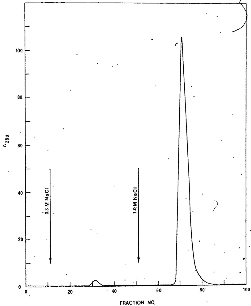
Crude uncharged tRNA in the 0.45 M NaCl buffer was chromatographed on a BD-cellulose column in the manner described. Lysine acceptor activity in the salt fractions was detected using the reaction mixture given in Table 5. The presence of lysine tRNA in the ethanol fractions was determined in the same way except that 1 ml fractions were previously dialyzed against the 1.2 M NaCl buffer to remove the ethanol.
